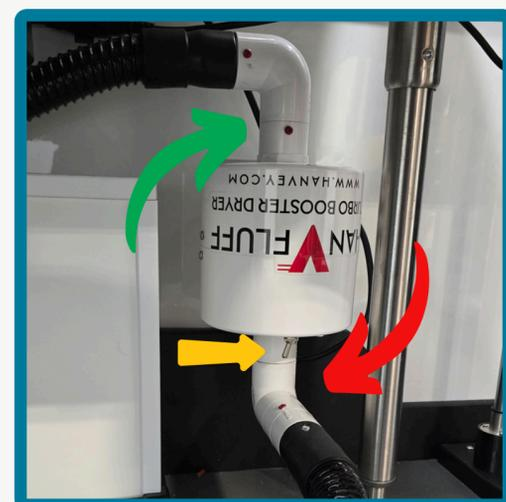
At this time, confirm that the metal switch is in the "ON" positioning and the extension cord is plugged in to the Red Switch Box in the Equipment Area. Then, secure the Fluff Dryer to the bracket. Your dryers are now in tandem!
